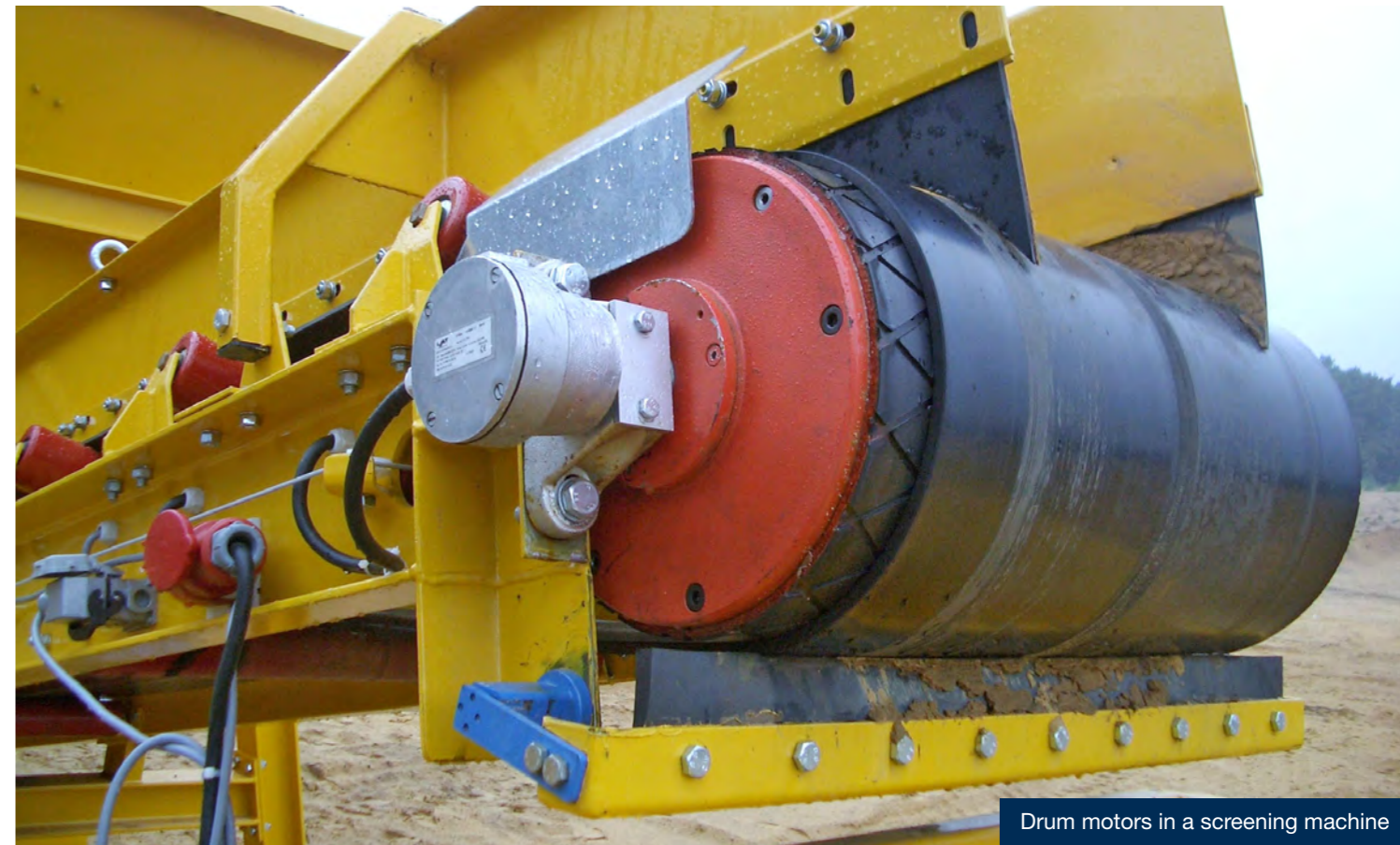
Drum motors in a screening machine
